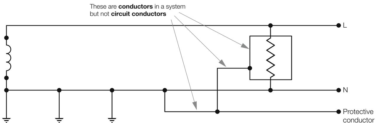
The combined neutral/earth conductor serves as both a neutral and a protective conductor and is therefore a **circuit conductor** as well as a **conductor in a system**
